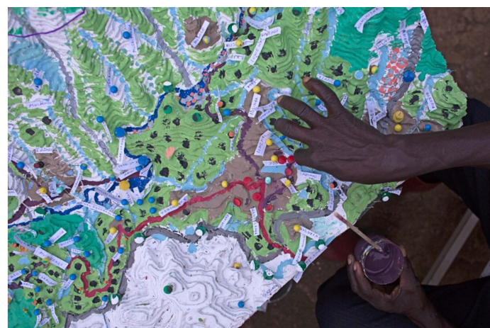
Figure 5 • The model is enriched with color codes, pins, and labels following a legend collectively defined by community members. Source: Riccardo Pravettoni and The Rainforest Foundation Norway [58].
